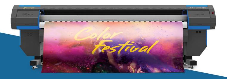
Neptune HQ, the high-speed Industrial grade eco-solvent printer is built for speed & quality. At a speed of 46 sqm/hr, Neptune HQ is engineered for highest quality of vinyl and flex printing with eco solvent inks. The 3.2 mtr eco-solvent printer based on industrial grade jetting assembly ensures accuracy at high speed.
